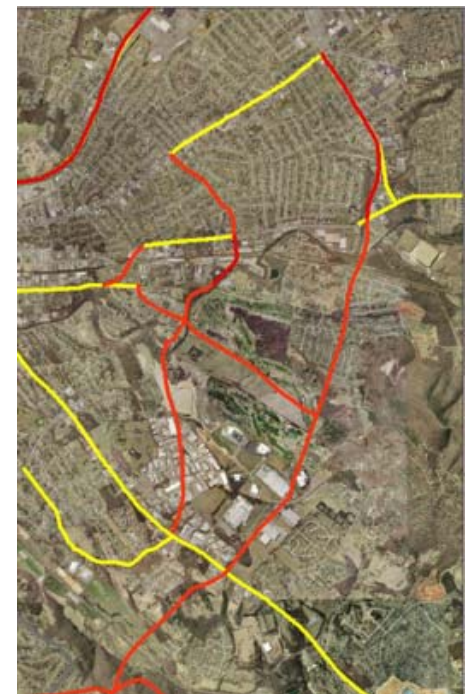
Thoroughfare Study: new terrain roadways proposed in past 30 years (red) and current model deficiencies (yellow)
